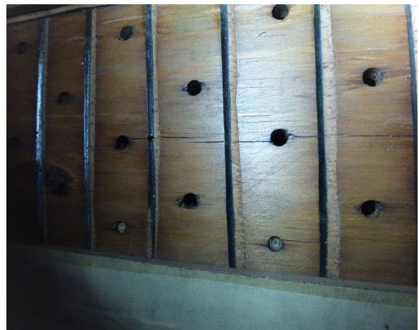
Cracks in Swell soundboard
