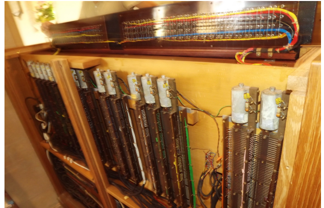
Inside 1963 console showing electro mechanical switching and piston wiring loom
