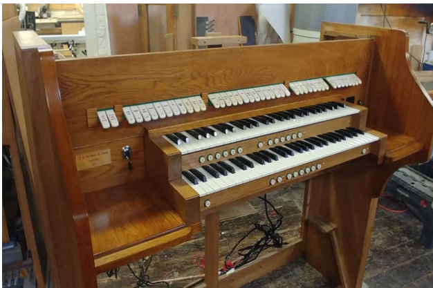
Workshop refurbishment - new keyboards and pistons fitted
