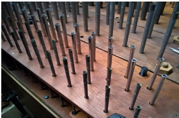
New Pipework for top of Great Mixture
