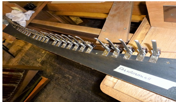
New pedalboard electrical contacts fitted
