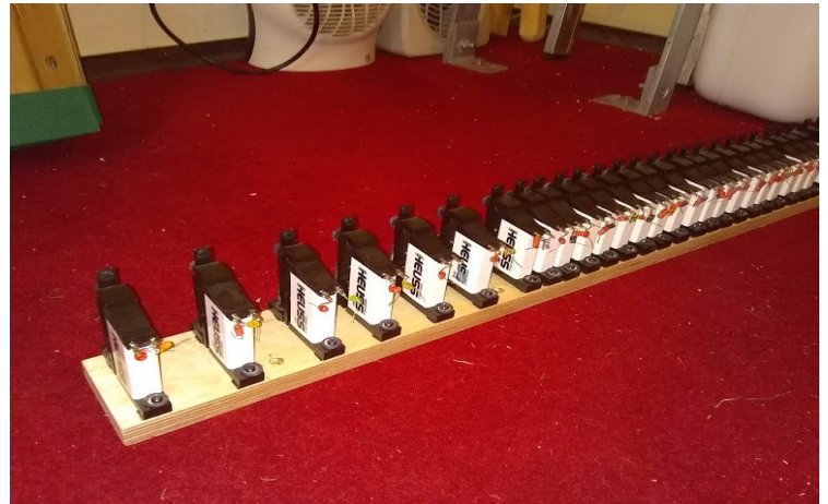
New direct electric action magnets set up for fitting to Swell Soundboard
